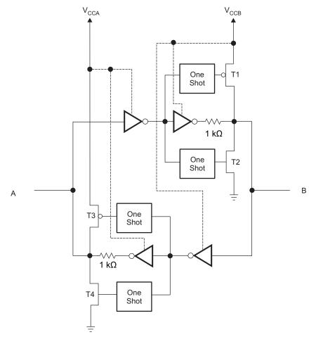
Figure 1. Architecture of TXB0302 I/O Cell
